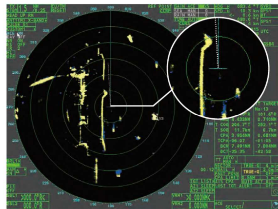
Automatic Clutter Elimination (ACE) ON
